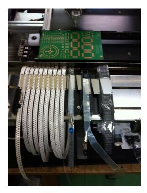
Cut tape blocks consist of 8mmx5, 12mmx4 and 12mmx2+16mmx2+24mm etc. and customer can choose them as required.
