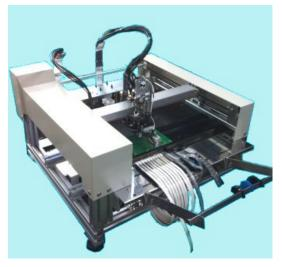
Handy full automatic pick & placer. It assumes approx 1000 chips per day production so it is suitable for prototyping and bread board assembly. PPP 1 model includes built in Vac pump so just mains power is necessary so easily set up any places just next to designer's desk.
