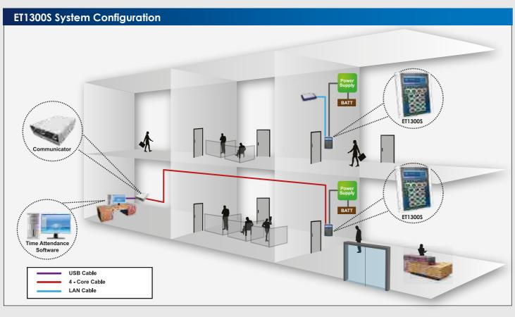
ET1300S LAN Configuration #16 #1 #2 #3 Communicato Time Attendance Software ET1300S ET1300S ET1300S ET1300S Maximum up to 16 units of ET1300S per bus (1KM) ET1300S WAN / LAN ET1300S
