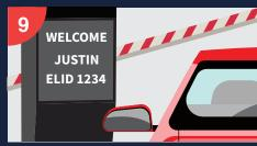
Display recognition information on screen and lift barrier gate.
